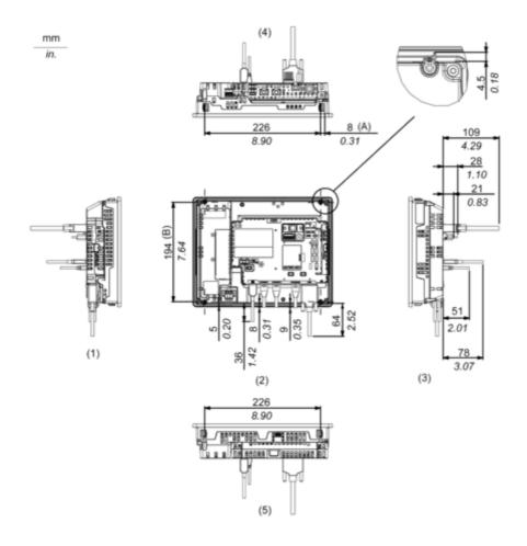
(A) Rotation area of the fastener(B) Pitch of the center of installation fastner screws
